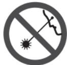
Do not direct the laser beam at persons or animals and do not stare into the laser beam yourself. This tool produces laser class 2M laser radiation and complies with 21 CFR 1040.10 and 1040.11 except for deviations pursuant to Laser Notice No. 50, dated June 24, 2007. This can lead to persons being blinded.
